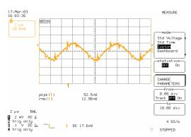
iHA48060A012V-001 Typical Output Ripple at nominal Input voltage and full load with external capacitors 47uF+1uF+0.1uF at Ta=25 degrees
